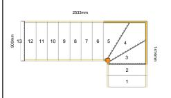
Winder Tread Material: Individual Rise: Going: Overall String Width: Nosing Style: Assembly: Est. Delivery Date: 22mm MDF Treads 200mm 222.12mm 900mm Half Round Assembled from 22 Feb 21 to 24 Feb 21
