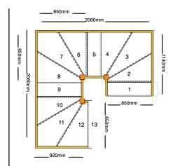
String Width Flight One: 850mm String Width Flight Two: 850mm String Width Flight Three: 850mm String Width Flight Four: 850mm Direction Turn One: Left Direction Turn Two: Left Direction Turn Three: Left Number of Treads in Flight One: Number of Treads in Turn One: 3 Number of Treads in Flight Two: Number of Treads in Turn Two: 3 Number of Treads in Flight Three: Number of Treads in Turn Three: 3 Number of Treads in Flight Four:
