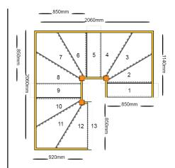
String Width Flight Two: 850mm String Width Flight Three: 850mm String Width Flight Four: 850mm Direction Turn One: Left Direction Turn Two: Left **Direction Turn Three:** Left Number of Treads in Flight One: Number of Treads in Turn One: 3 Number of Treads in Flight Two: Number of Treads in Turn Two: 3 Number of Treads in Flight Three: Number of Treads in Turn Three: 3 Number of Treads in Flight Four: 0
