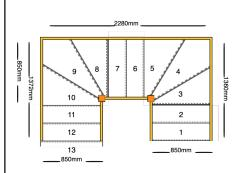
Stair Type: Double **Building Regulations:** UK String Width Flight One: 850mm String Width Flight Two: 850mm String Width Flight Three: 850mm Number of Treads in Flight One: 2 Turn One Direction: Left Number of Treads in Turn One: 3 Number of Treads in Flight Two: 2 Turn Two Direction: Left 3 Number of Treads in Turn Two: Number of Treads in Flight Three:
