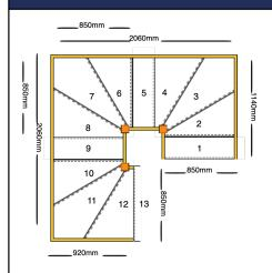
Stair Type: Triple **Building Regulations:** UK String Width Flight One: 850mm String Width Flight Two: 850mm String Width Flight Three: 850mm String Width Flight Four: 850mm Direction Turn One: Left Left Direction Turn Two: Direction Turn Three: Left Number of Treads in Flight One: Number of Treads in Turn One: 3 Number of Treads in Flight Two: Number of Treads in Turn Two: 3 Number of Treads in Flight Three: Number of Treads in Turn Three: 3 Number of Treads in Flight Four: 0
