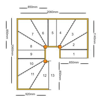
Direction Turn One: Left Direction Turn Two: Left Direction Turn Three: Left Number of Treads in Flight One: Number of Treads in Turn One: 3 Number of Treads in Flight Two: Number of Treads in Turn Two: 3 Number of Treads in Flight Three: Number of Treads in Turn Three: 3 Number of Treads in Flight Four:
