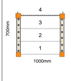
Straight Staircase UK 830mm 4 Closed tread construction 32mm Redwood Pine (Furniture Grade) 22mm MDF Treads 9mm MDF Risers 207.69mm 230.66mm 1000mm Half Round 90mm x 90mm Pine 90mm x 90mm Pine 90mm x 90mm Pine 90mm x 90mm Pine PSE Newel 90mm x 90mm Pine Yes Yes Yes 1500mm Softwood Stop Chamfered Assembled from 26 Feb 21 to 02 Mar 21 Ground To First Section 2
